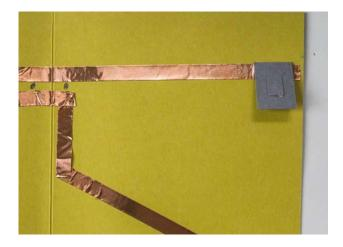
The last piece of tape runs vertically from the switch to the battery. At the battery end, you will make a tab to place over the battery.
