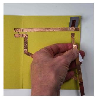
• Create a tab with the remainder of the tape by folding the end back and pressing the adhesive surfaces together.
