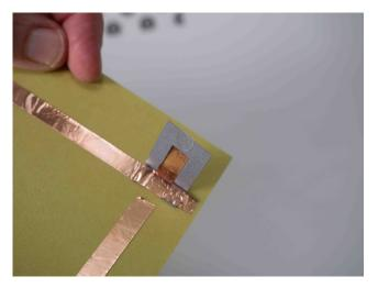
• Press any wrinkles out of the copper tape using the the tool you've chosen with a smooth flat edge.
